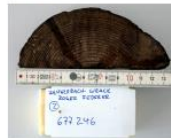
W-178550 LdNr 677246, DateEnd: 1789 UnReliable, Fichte (Picea abies (L.) Karst. / PCAB), NR/Rings 29, Missing
